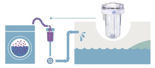
The Filtrol is an affordable, easy to install filter. It stops microfibers as they leave your washing machine and makes it easy to put them into the trash. The Filtrol works flawlessly and you can start saving yourself money and help prevent a majority of fibers from being released into wastewater/sewer treatment plants where they can lead to additional issues.
